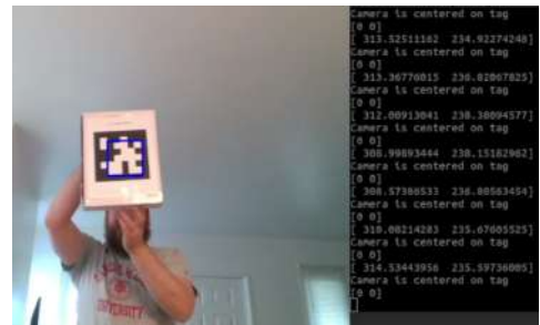
Figure 15: Testing Pan-Tilt Control
