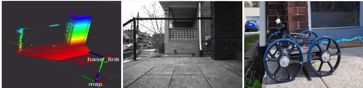
Figure 11: Left: Generated Point Cloud, Center: Rover View, Right: Final Position
