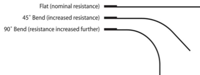
Figure 1. Flex sensor resistance changing with angles
