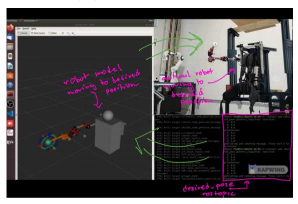
Figure 1.1: Robot arm moving to goal pose video screenshot
