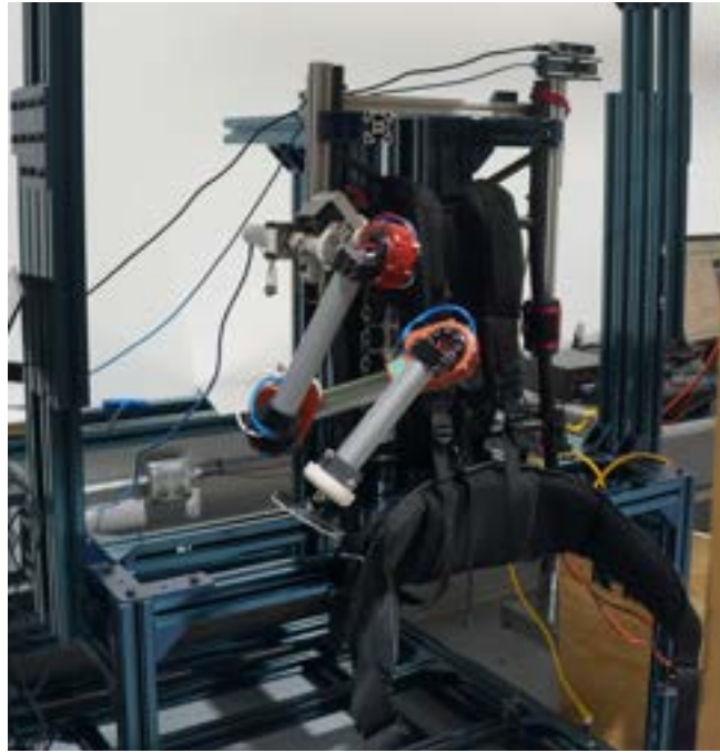
Figure 11 - Manufactured State of COBORG, Mounted onto Testing Frame
