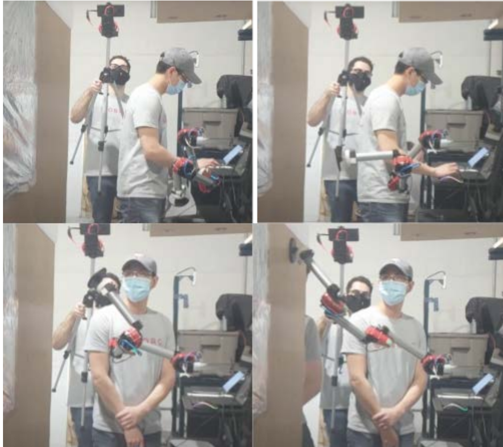
Figure 12 - Actuated Manipulation Push Out Process Screenshots: compact/home position (top left), ready pose (top right), X-offset to push out (bottom left), final goal position (bottom right)
