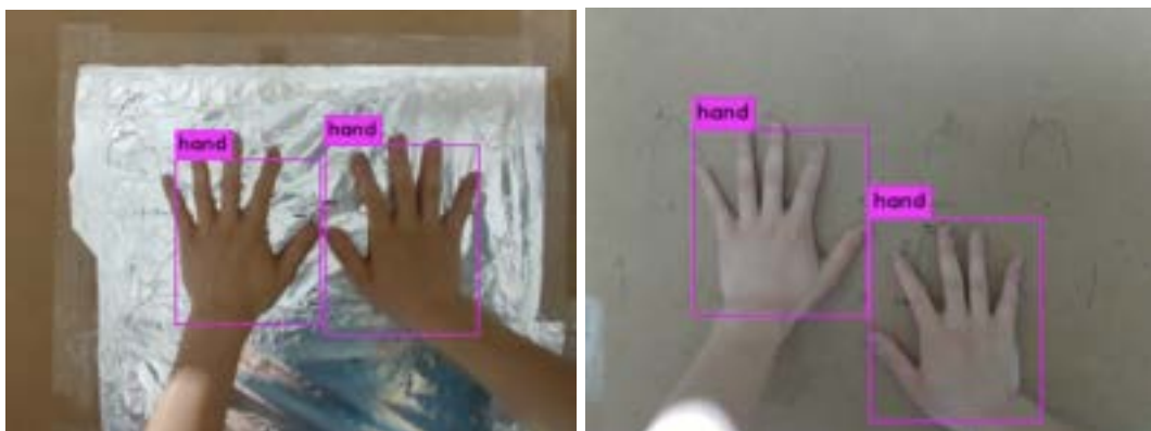
Figure 9 - Sample Outputs for 2D Hand Detection Results
