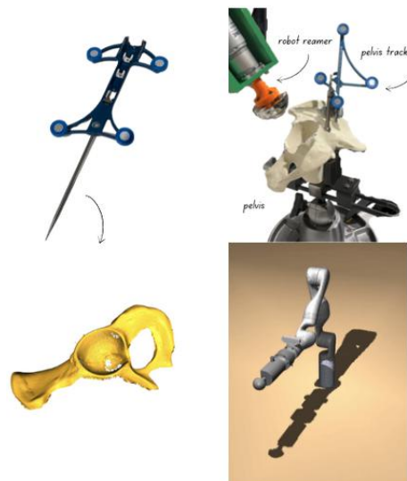
Figure 7: The various system inputs (i) Registration Probe (ii) Pelvis EE Marker (iii) Pelvis CAD model (iv) Robot Arm CAD model
