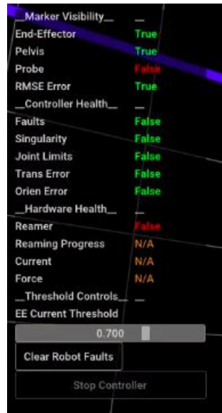
Figure 15: Watchdog critical parameters displayed on the UI
