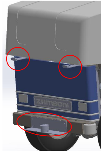
Figure 4: Front face of the Zamboni resurfacer with mounts installed
