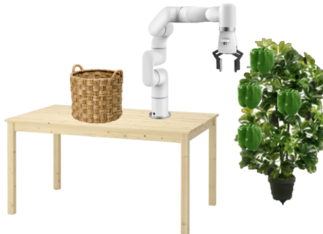
Figure 1 – Depiction of the testbed setup with the xArm 6 and a fake plant with real peppers
