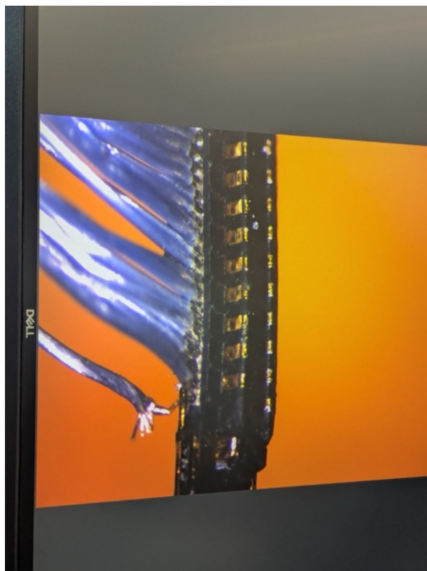
Figure 2: Broken data cable, under a soldering microscope.
