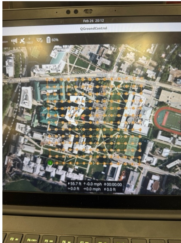
Figure 1: Path Planner for searching the Geofence Zone on QGroundControl
