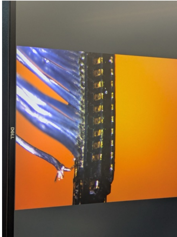
Figure 2: Broken data cable, under a soldering microscope.
